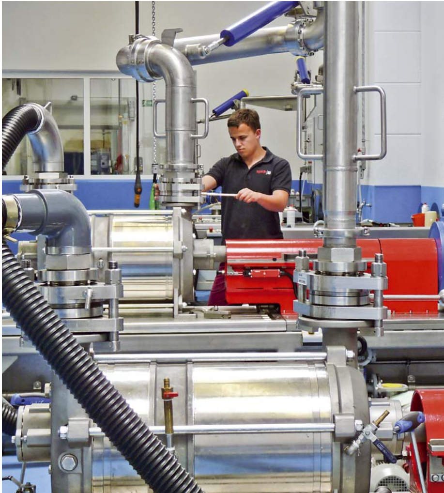
Computer-controlled and fully automated test stands for vacuum pumps on the premises of Speck in Roth. Measuring of hydraulics, power requirements and vibrations. Test of inlet pressures up to 5 mbar and suction capacities up to 2000 m 3 /h..
