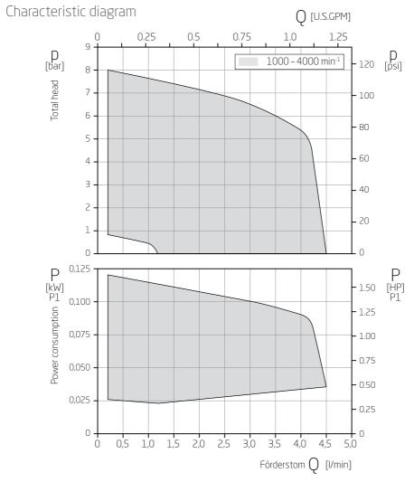
Every operating point can be reached within these characteristic diagrams by setting different drive parameters.
