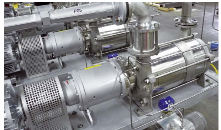
VHCM (ChemTAL) liquid ring vacuum pump as per TA Luft with a pump monitoring system used for solvent recovery.
